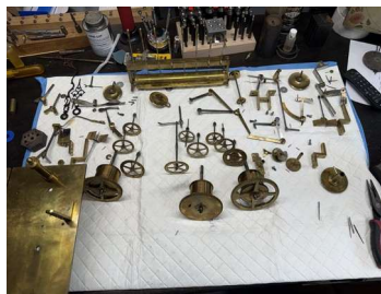
Complete disassembly permits inspection of every train and control component.
